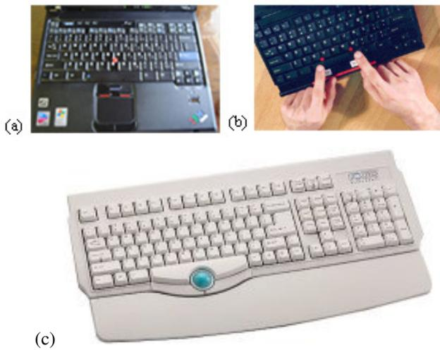
**Figure 2. Examples of Integrated Input Devices: (a) Keyboard with integrated Track point and Touchpad, (b) Keyboard with two integrated Track points (c) Keyboard with integrated Trackball.**
