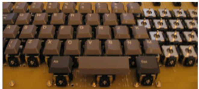
Figure 1. The Joystick Keyboard uses mini-joystick sensors to detect key press and sense multiple degrees of freedom.
